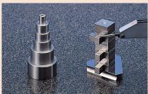
Using a base, plain jaws, tie rods, flat head screws and gauge blocks, a gage was constructed to enable rapid comparison measurement of a stepped workpiece. (Sample workpiece)
