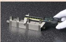
Using plain jaws, tie rods, knurled head screws and gauge blocks, a gage was constructed to enable rapid comparison measurement of a stepped workpiece. (Sample workpiece)
