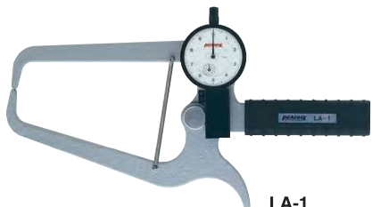
LA-1 Graduation: 0.1mm Range: 0-80mm Throat depth: 120mm
