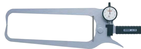
LA-23 Graduation: 0.1mm Range: 0~80mm Throat depth: 300mm
