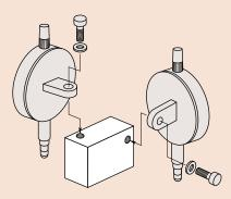
Note 1: If back lids are replaced when using a waterproof or dustproof model, the water resistance will not be guaranteed. Note 2: When installing to **297XTB** Series, separately prepare 4 fixing screws (**546666** Self-tapping screw only for plastic). Do not apply a tightening torque of more than 20 N-cm in order to avoid stripping the screw threads.
