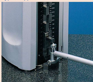
Bore gage zero-setting
