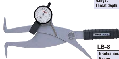
LB-5 Graduation: 0.01mm Range: 20-40mm Throat depth: 150mm
